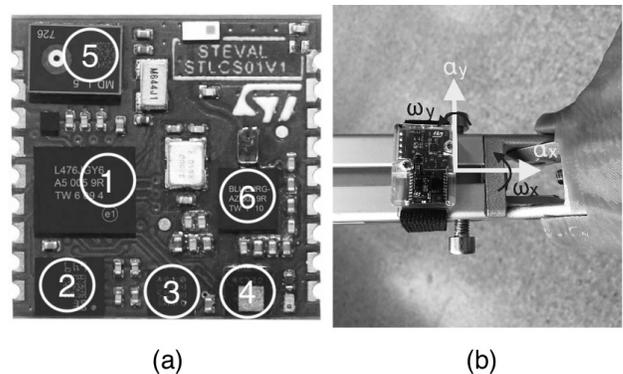
Fig. 2. Illustration of the STEVAL-STLCS01V1 (SensorTile) (a) The 13.5 x 13.5 mm grove board with the sensor markings from Table III [34]. (b) Shows the complete wrist sensor assembly and correct placement on the Fall Simulator. The axes indicate the orientation in which the sensor records them. The indicative values are those of the accelerometer  $\alpha_x$ ,  $\alpha_y$ , and the gyroscope  $\omega_x$ ,  $\omega_y$ .
