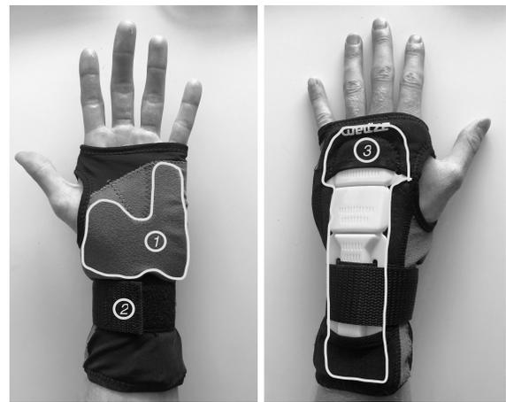
Fig. 6. Snowboard wrist protectors: (1) 0.7 mm thick impact protection on the palm of the hand (2) Strap for fastening (3) Shell to protect against wrist bending
