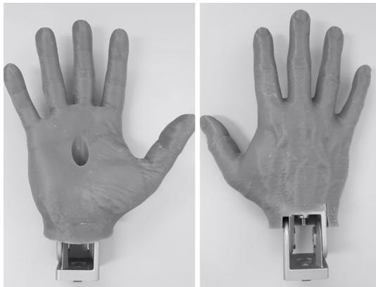
Fig. 4. Urethane cast hand which is screwed to the joint through the palm of the hand in the direction of the wrist.
