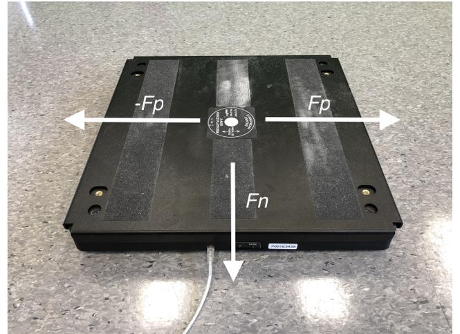
Fig. 3. Force plate: Arrows show in which directions the forces are absorbed ( $F_n$  = normal force;  $F_p$  = parallel force). The drop structure falls in the longitudinal direction to the parallel forces  $F_p$ .
