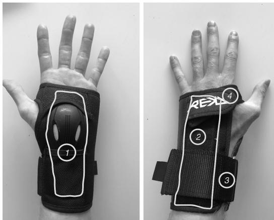
Fig. 5. Inline hand protector: (1) Protective shell (2) Shock-absorbing 6 mm thick foam padding (3) Strap to attach to wrist (4) Strap to attach to palm
