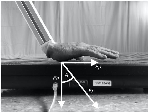
Fig. 7. Representation of the impact force.  $F_p$ =parallel force,  $F_n$ =normal force,  $F_r$ =resultant force,  $\theta$ =angle of resultant force.
